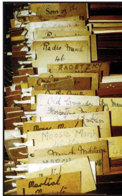
Figure 2. Dozens of folding cardboard book music masters hung from racks in the Chiappa firm’s music library. Victor’s father Ludovico arranged and punched the music starting in 1918. Titles shown here are 46-key books. Chiappa built many 46-key instruments using the Gavioli scale.
